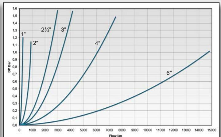
Pressure drop for 1" to 6", scale 0-15000 l/min.
