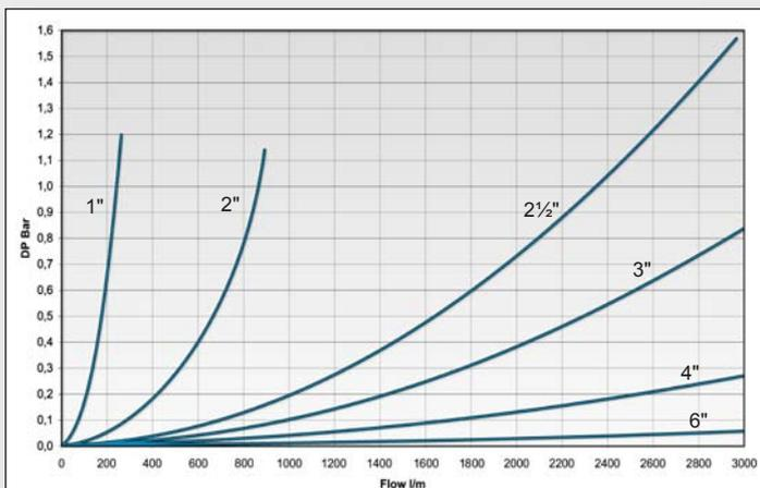
Pressure drop for 1" to 6", scale 0-3000 l/min.
