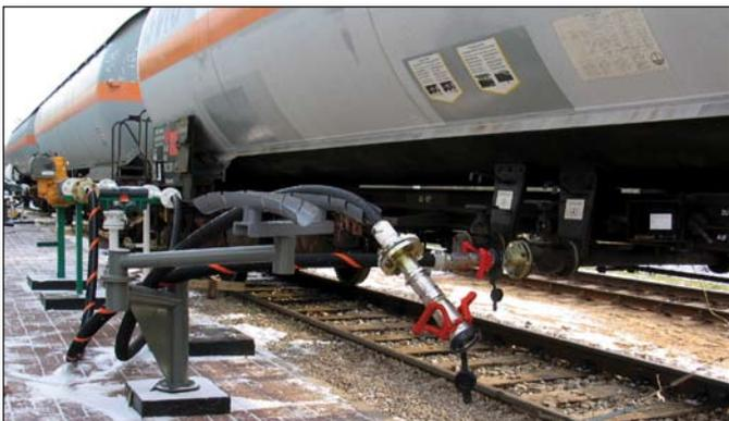
TODO-GAS® DRY-BREAK® couplings are designed specially for the safe and efficient handling of LPG in both liquid and vapour phases. Certified towards European Directive 97/23/EC (P.E.D.) category II.
