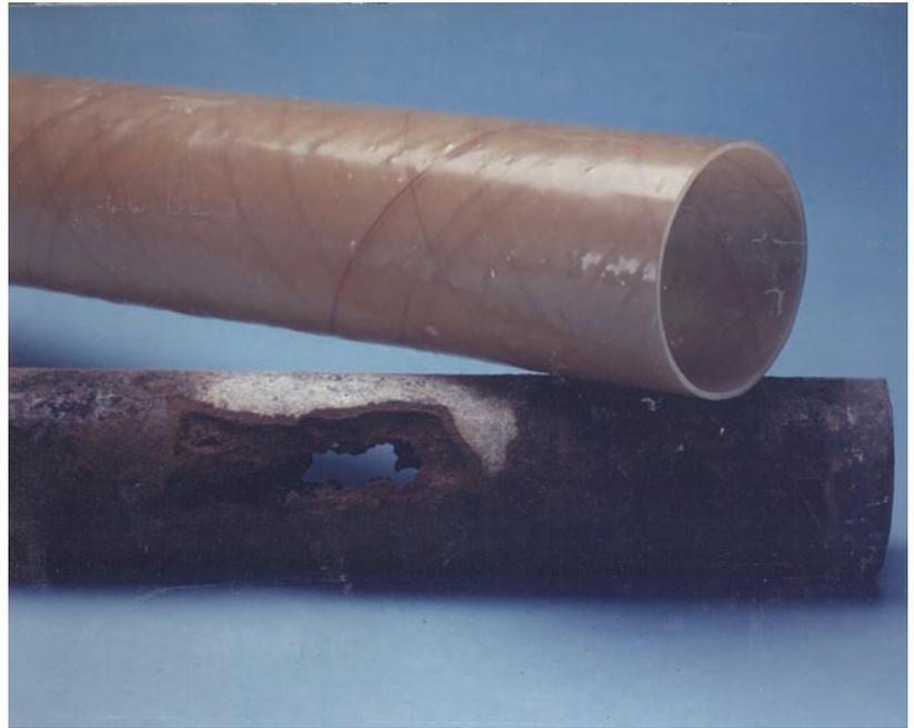
Fiberglass has a long corrosion-free service life and requires no coating or cathodic protection.
