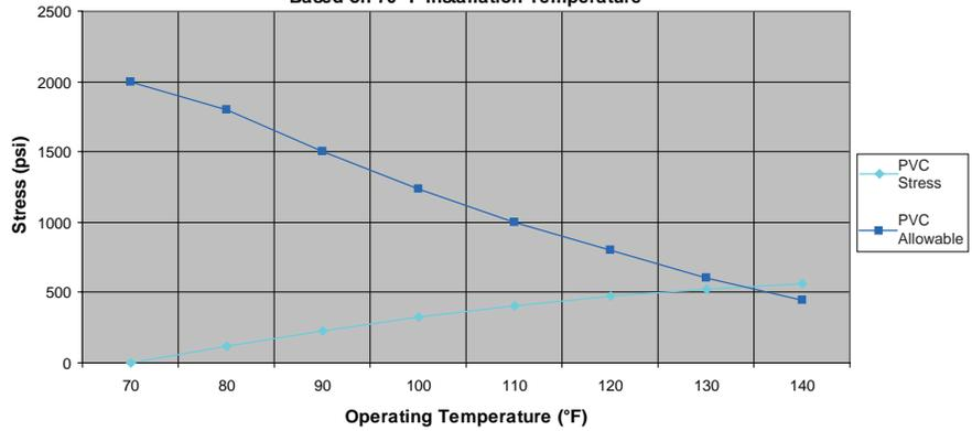
Figure 6 - Steel Pipe Restrained Thermal End Load Stress Based on 70° F Installation Temperature
