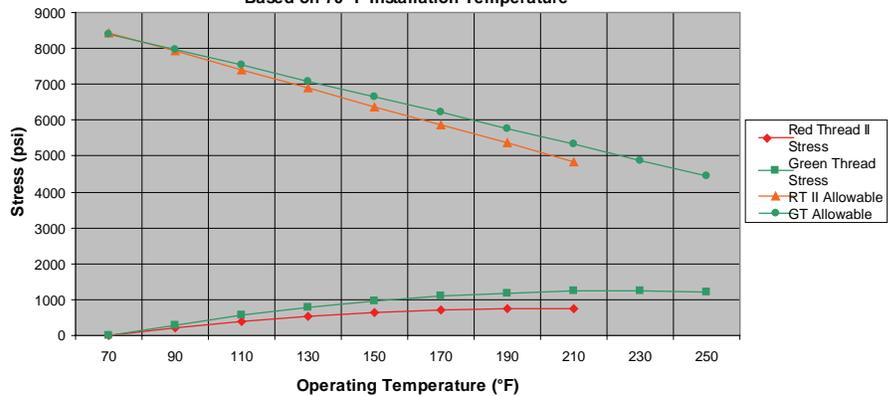
Figure 5 - PVC Pipe Restrained Thermal End Load Stress Based on 70° F Installation Temperature
