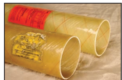
Old vs New - Pipe in the foreground was installed in 1973 and removed 27 years later when the station closed.
