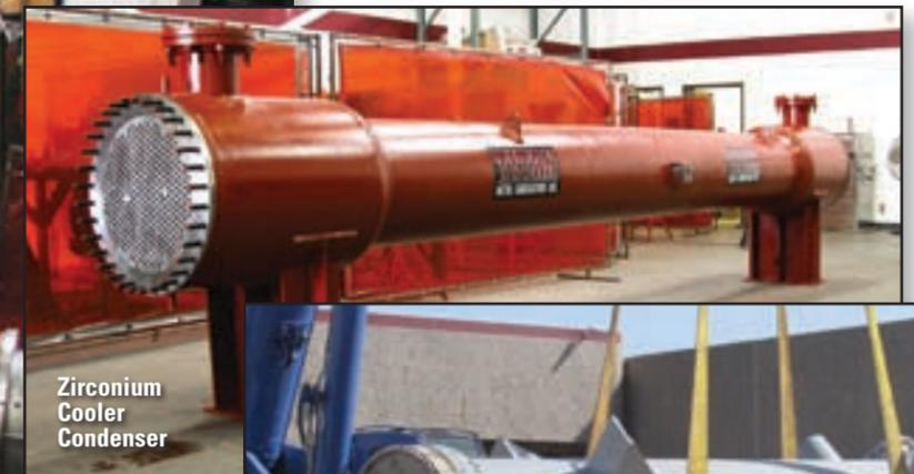
Zirconium Cooler Condenser
