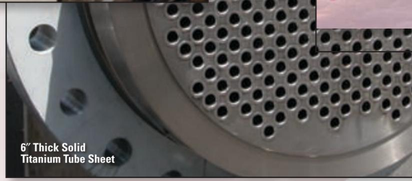
6" Thick Solid Titanium Tube Sheet
