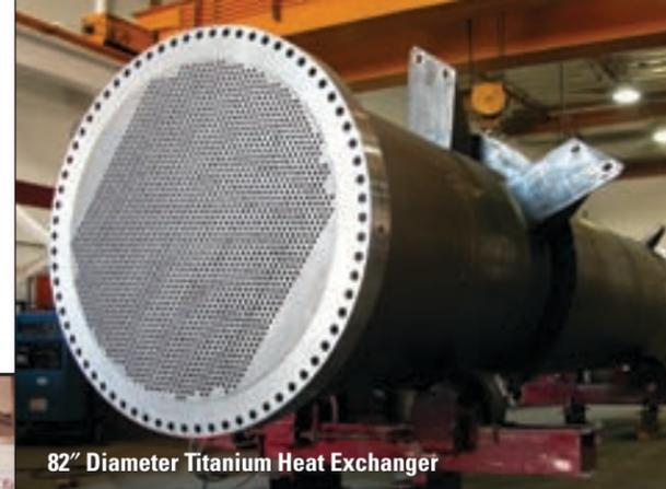
82" Diameter Titanium Heat Exchanger
