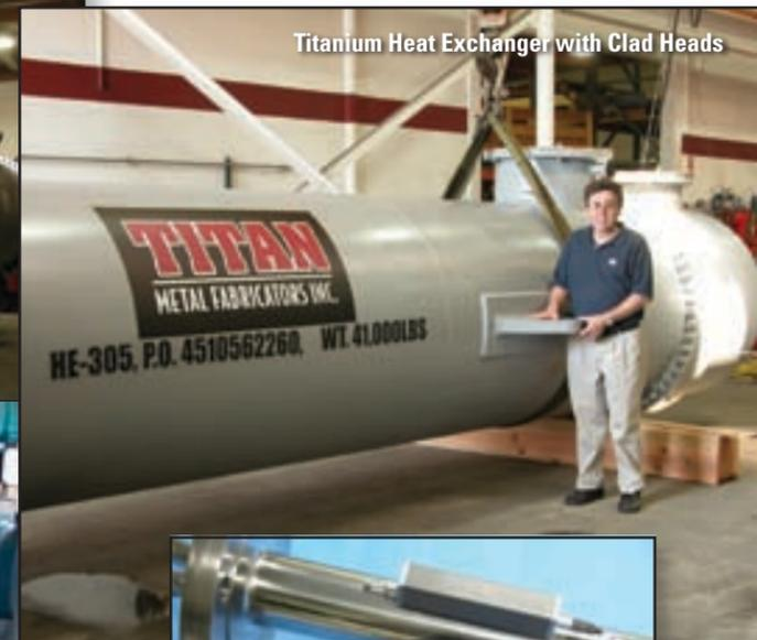
Titanium Heat Exchanger with Clad Heads
