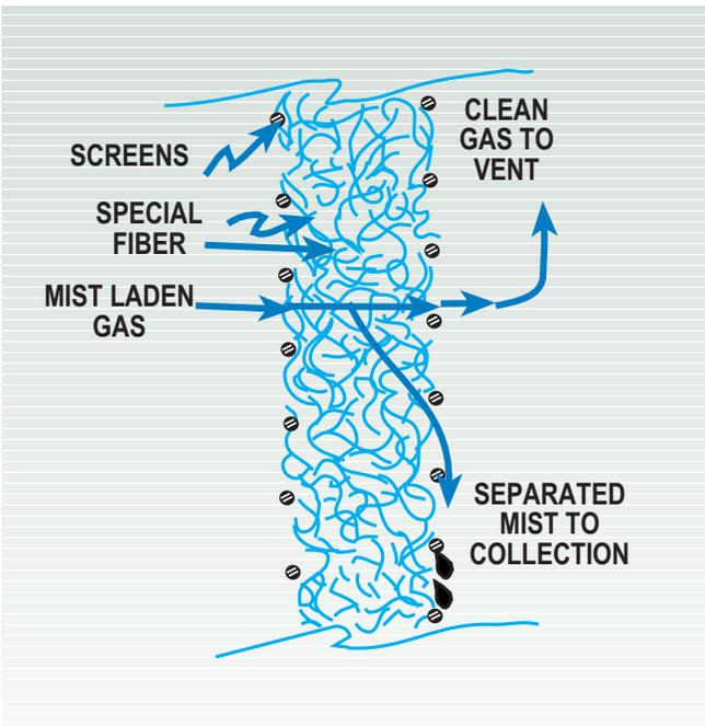
Figure 1. Single stage vertical FLEXIFIBER<sup>®</sup> mist eliminator
