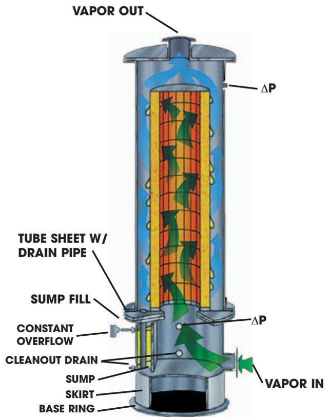
**Figure 4. FLEXIFIBER® mist eliminator for lube oil tank vents on gas or steam turbines.**
