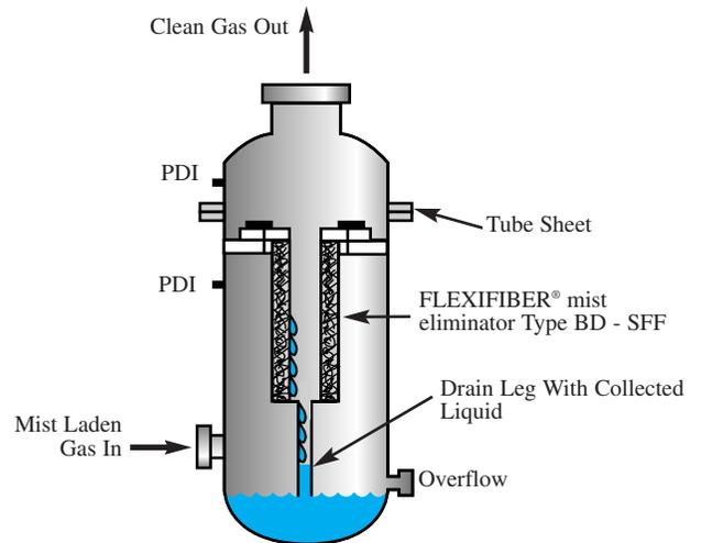
**Figure 3. Typical FLEXIFIBER® mist eliminator assembly (forward flow installation).**
